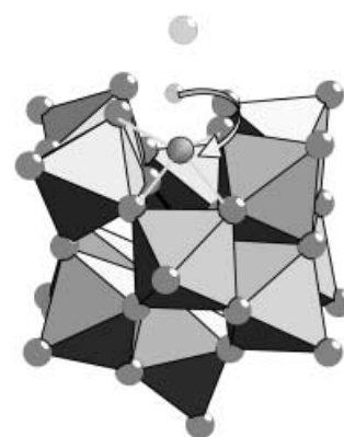
Figure 15. Schematic representation of a partially decomposed Keggin anion (lacunary Keggin anion) as a model for the catalytically active species in heteropolyoxomolybdate partial oxidation catalysts.
